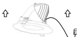
Fig.3. Hold the luminaire and the driver up to cut-out with the springs being held vertically.
